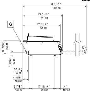
EQ = Equipotential screwG = Gas connection
